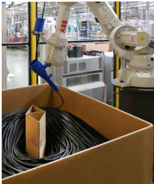
Robot-controlled insertion of the profile into bulk packaging
