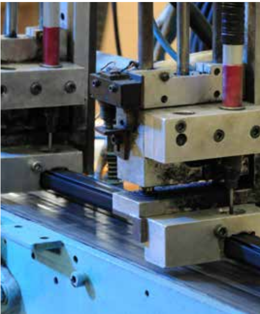
Drilling device for vent holes
