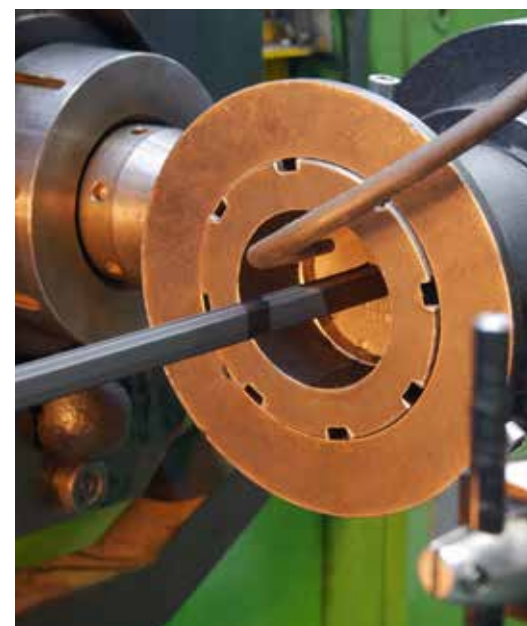
Extrusion die with emerging rubber profile
