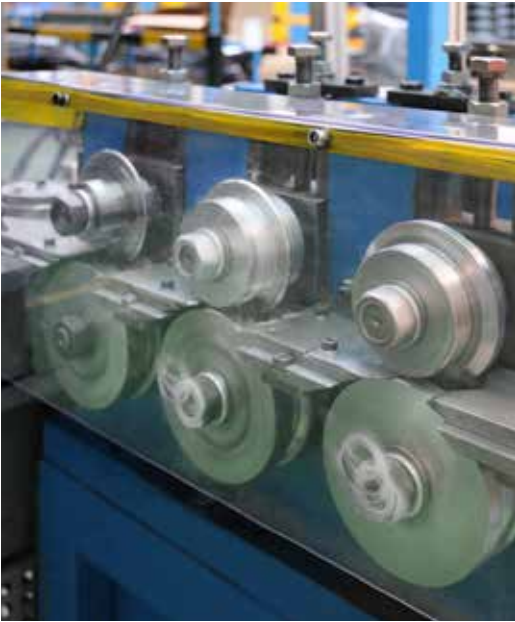
Bending roller set for profiling
