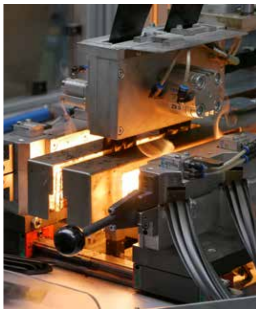
PE film bonding for rings and frames
