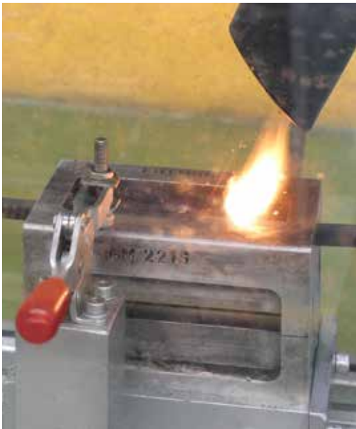
Laser marking of the rubber profile according to customer requirements
