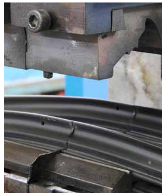
EPDM film vulcanization for rings and frames
